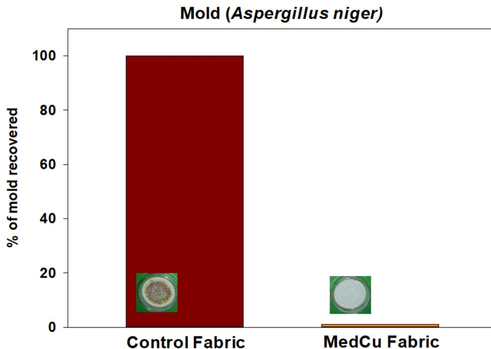
**Figure 4: MedCu fabrics and Control Fabrics were inoculated with  $2 \times 10^6$  *Aspergillus niger* spores. After 24 hours of incubation, the mold spores were recovered and plated on petri dishes. While mold recovered from the Control fabric grew readily, no mold grew from the MedCu fabrics (example shown in inserts).**
