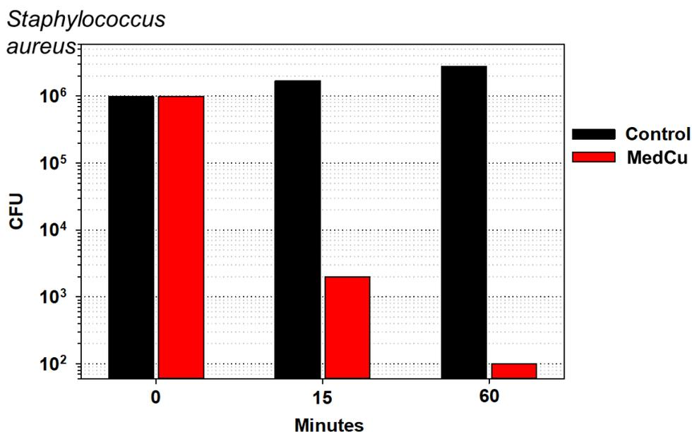
**Figure 3. MedCu copper oxide impregnated fabrics kill more than 99% of the tested bacteria during 15 minutes of exposure of the bacteria to the mask surface.**
