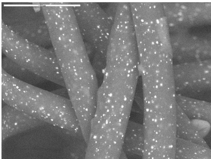
**Figure 1. Scanning electronic microscope image of polypropylene fibers impregnated with copper oxide microparticles.** The white dots are copper oxide microparticles. The particles are physically impregnated in the polymeric matrix.
